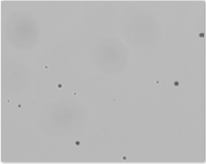
Etch-pits by thermal neutron
