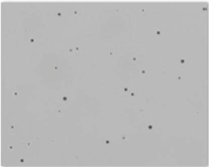
Etch-pits by Cf-252 source
